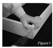
**Step 1 -** Screw Cross Brace to Side Rail. (See Fig. 1) The Sievers Benchwork stamp will face the inside of the section. **NOTE:** A blue pencil line indicates the top edge of each piece.
